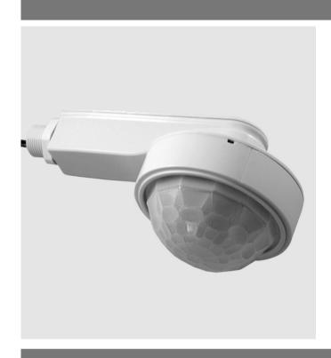
The EBDHS-MB-DNET1 is a combined passive infrared (PIR) motion sensor and photocell designed to be part of a DALI network. The EBDHS-MB-DNET1 is a high sensitivity PIR detector suitable for high bay applications, such as warehouses and factories, and where high detection sensitivity is needed. It is specifically designed for mounting onto a batten style luminaire.
